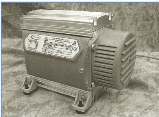
Figure 13. Vacuubrand MD 1 Vario Diaphragm Pump
