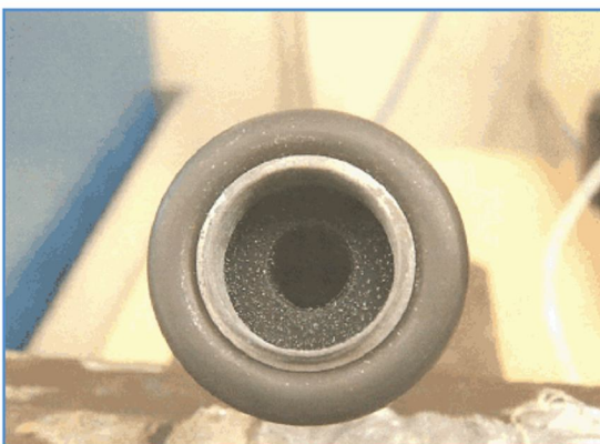
Figure 27. Iwata ISP 90 Filter Inlet Showing Corrosion
