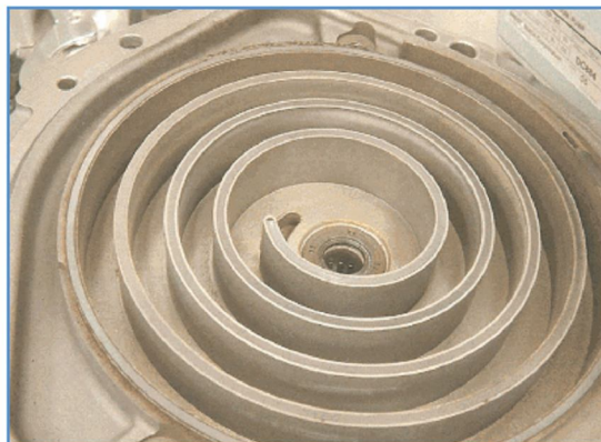
Figure 26. Iwata ISP 90 Fixed Scroll showing Particulate
