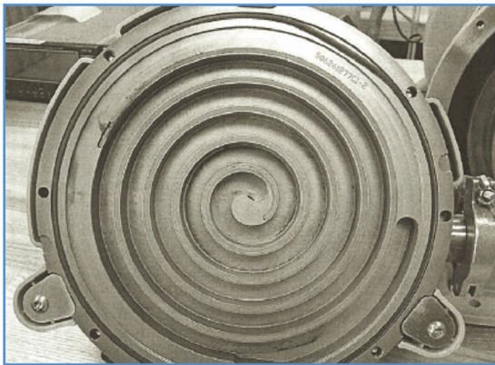
Figure 21. Edwards XDS 5 Fixed Scroll Showing Particulate
