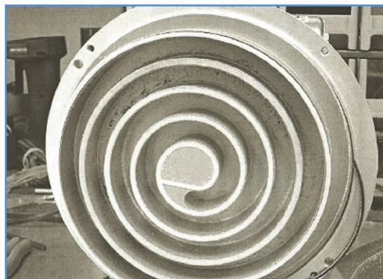
Figure 24. Varian SH 100 Orbiting Scroll showing Particulate and Uneven Wear
