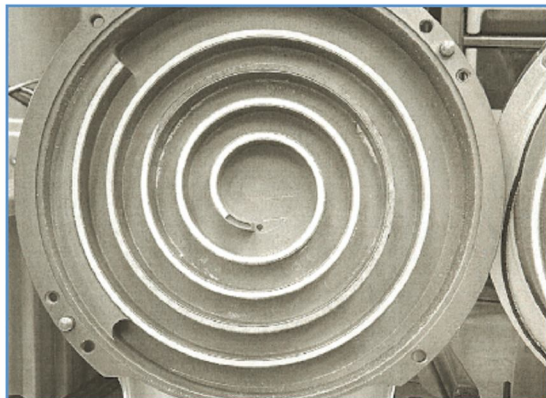
Figure 23. Varian SH100 Fixed Scroll showing Particulate and Uneven Wear
