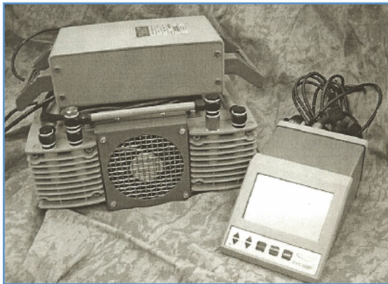
Figure 6. Vacuubrand MD 4 Vario Diaphragm Pump
